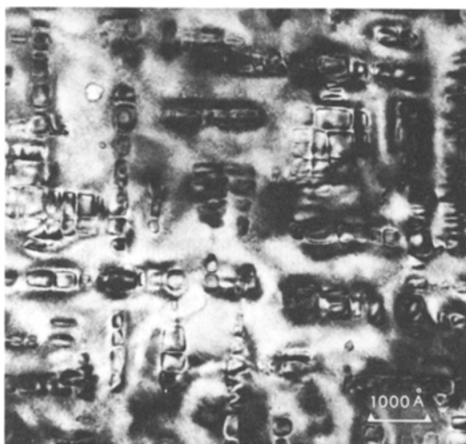
Figure 7 Cu-31.6 Ni-1.7 Cr alloy aged for 200 h at 650° C showing tendency of cuboids to congregate into rafts and rods.
