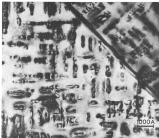
Figure 6 Cu-31.6 Ni-1.7 Cr alloy aged for 25 h at 700° C showing the absence of precipitate-free zones at grain boundaries.
